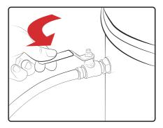
Open the vacuum valve on the chamber which connects it to the vacuum pump by turning it to the inline position.
