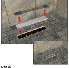
Various options are available to accessorise the linear drain including a fileable drain cover option. These are installed in the same way as above; just adjust the black plastic height adjustment nuts to suit.
