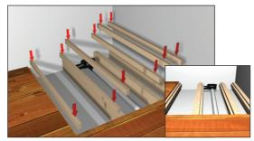
All exposed joists will now need a batten running along the inside of the joist to accommodate the new plywood low level floor. Measure the length of the exposed joist taking into account any obstructions. Cut some timber batten to length and screw at approximately 150mm intervals to the inside of all joists 18mm below the top of the joists.
