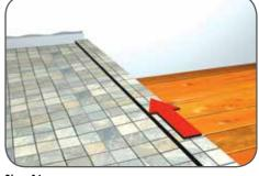
After tiling the base of the shower area, we recommend that you add a further narrow border of tiles approximately 30mm to 40mm wide, along the top of the outside edge to act as a water retainer, stopping water running out of the shower area. The tiling aid can now be removed and disposed of.
