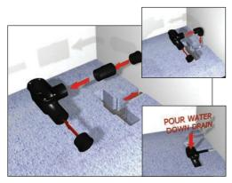
Note: All solvent joints should be cleaned with an appropriate solvent weld cleaner prior to using solvent adhesive.
