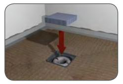
13. Place the Disposable Tiling Aid, available separately, into the shower drain hole on the Shower Tray. The Tiling Aid provides the edge that needs to be tiled up to whilst protecting the Shower Drain from debris.
