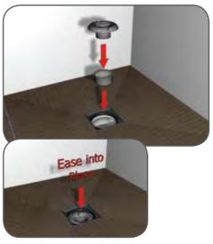
5. Put your fingers through the drain hole in the Shower Tray. Push down on the Shower Tray and pull the Shower Drain upwards until it clicks into place into the drain hole in the Shower Tray. 6. Ease the Shower Drain Internal Bowl into the Shower Drain. Ease the Shower Drain Internal Dome into the Shower Drain. When you have finished you can remove the protective gloves and eye and breathing protection.
