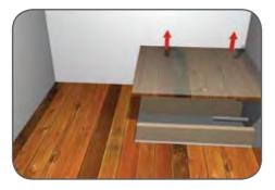
1. Remove flooring as necessary to carry out works to the waste pipe. Please note that if there is a joist in the way of the Shower Tray you will need to consult a professional joiner or structural engineer for advice.
