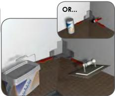
10. Place the Waterproofing Internal Corners into the internal corners of the shower area and push firmly into the tape sealer. Apply a further thin layer of tape sealer over the edges of the waterproofing internal corners.
