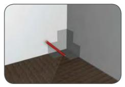
8. Temporarily place the Waterproofing Internal Corners into position and mark around them with a pencil. Once you have marked they can be set aside for the moment. This is to show where you need to apply the tape sealer.
