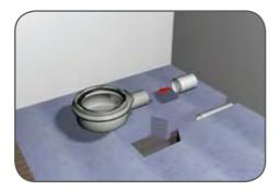
3. For water to drain away properly, the waste pipe must have a fall of at least 3cm per metre. The waste pipe must be properly supported to hold its own weight and that of the Shower Drain. Connect the Shower Drain to your waste pipe using a 2" solvent weld connector. Once the solvent weld has set; pour water down the drain to check that the waste is not blocked and that there are no leaks.
