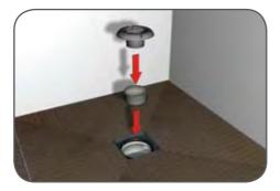
Ease the Shower Drain Internal Bowl into the Shower Drain. Ease the Shower Drain Internal Dome into the Shower Drain. When you have finished you can remove the protective gloves and eye and breathing protection.
