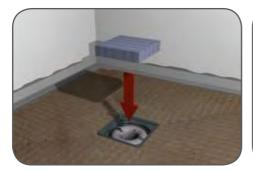
13. Place the Disposable Tiling Aid, available separately, into the shower drain hole on the Shower Tray. The Tiling Aid provides the edge that needs to be tiled up to whilst protecting the Shower Drain from debris.
