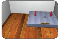
Place the Substrate Element into position and bed down onto the adhesive cement. Check that the Substrate Element is level in both directions using a suitable level.
