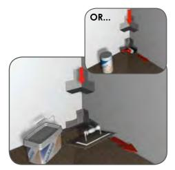
Note: Wear protective gloves, eye and breathing protection. Using the non-notched end of the notched adhesive trowel, apply a thin layer of tape sealer to the internal corners of the shower area, slightly bigger than the pencil line marked in Step 8.
