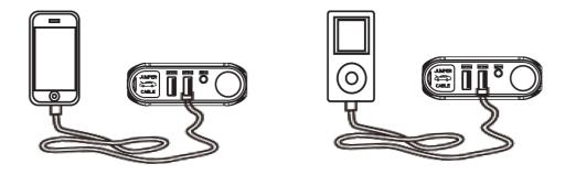
Connect the device you wish to be charged to the USB output port socket using an appropriate cable and depress the ON/OFF switch on the top of the unit. The blue battery status indicator LEDs on the face of the product will illuminate and charging will commence automatically.
