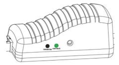
Upon successful starting the red and green LEDs will flash; the jump cable can now be disconnected. Remove the black (-ve) clamp first, followed by the red (+ve) clamp. Leave the vehicle engine running for a period after disconnection to allow battery to be recharged.
