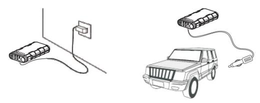
The device can be charged in two ways:
