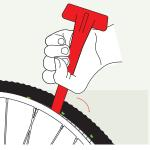
As you are locking pins into place, be sure to tuck in the tire edge into the rim as you go so that the tire sits flush in the rim channel. This will ensure a safe and smooth rolling tire.
