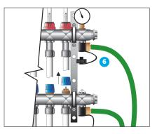
6 Fully loosen the protection cap from the first zone to be filled.
