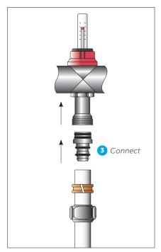
Connect the flow pipe to the ports on the upper manifold with the fittings supplied – the lower manifold may be removed to make this easier.
