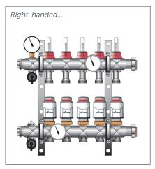
2 Remove the temperature gauges (these are a press fit), unscrew the boss and the blanking screw on the reverse.
