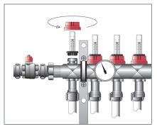
**3** Fully open all the flow adjusters on the supply (top) manifold by lifting and inverting the red locking collar which may then be used to turn the black collar fully anti-clockwise.
