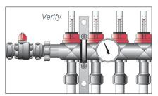
Note: Flow rates detailed on the A3 Manifold and Zone Information sheet are a minimum. The flow setting should be set as close to this level as possible, or slightly above.
