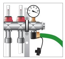
**13** Allow the pressure to rise to a maximum of 3 bar.
