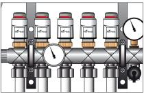
At this stage the blue protection caps can be replaced with actuator heads on each manifold port.
