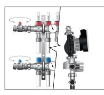
Close the isolating ball valves that are either connected directly to the manifold, or connected just before the Direct Mounted Pump Module.
