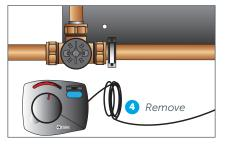
4 Remove the head from the blending valve on the pump module if fitted. Ensure the valve shaft and actuator motor are positioned correctly when re-assembling (see p.14–17).
