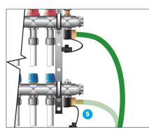
5 Similarly fix a suitable hose to the drain valve on the return (lower) manifold.
