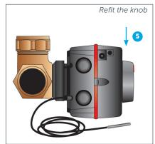
Refit the knob. The valve position 6 can now be aligned with the valve body motor by turning the knob clockwise or anti-clockwise with a slight downward force.
