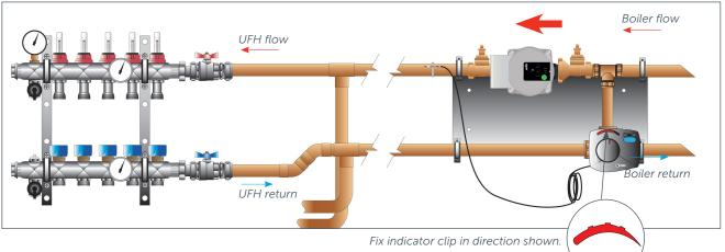
Important: Do not fit or power up the electric blending valve head at this point of the installation.
