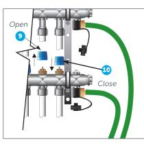
Tip: If the outflow is run into a bucket then air bubbles will be detectable.
