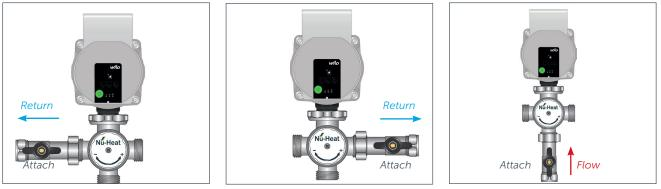
**3** Take the straight isolating value and attach to the left-hand side, right-hand side or bottom of the blending value as required.
