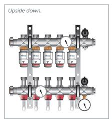
3 Refit the boss on the front of the rail and the blanking screw on the back. Refit the temperature gauges.
