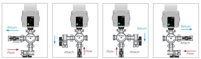
4 Attach the other isolating valve to the bottom of the temperature blending valve using the attached captive nut and rubber washer provided. The two valves must be pointing in the same direction.
