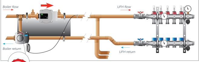
Fix indicator clip in direction shown. Important: Do not fit or power up the electric blending valve head at this point of the installation.
