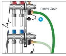
4 Remove the blanking cap from the filling valve on the flow (upper) manifold. Fit the hose connection nozzle (from the *Tools and Accessories Pack*), and connect a suitable hose from the mains water supply. Open the filling valve using the key on the blanking cap.
