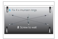
The **Remote Mounted Pump & Valve Module** should be screwed to the wall using the holes provided in the backplate.
