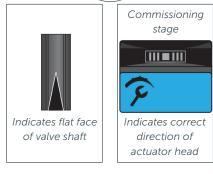
Adjust the flat face of the shaft on the blending valve to the position shown
