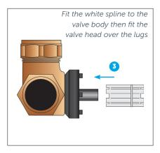
4 Fit the white spline coupling to the valve body and fit the valve actuator head over the lugs, be careful not to move the valve shaft or the knob from the mid position
