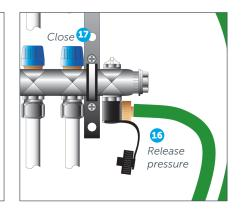
16 After testing, reduce the pressure to 1 bar-static by releasing the water from the drain valve on the return (lower) manifold.
