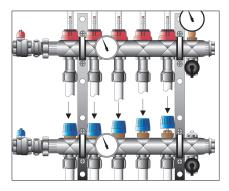
Isolate all zones by screwing down all the blue protection caps hand tight.
