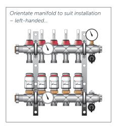
Unscrew the manifold-rail mounting clamps, turn the manifold to the correct orientation and re-fit the mounting clamps.
