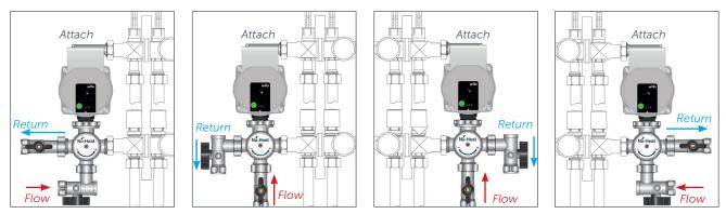
**5** Take the elbowed pump connector and attach this to the top of the pump with the free end pointing in the opposite direction to the isolating valves.
