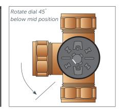
Use the plastic knob provided to turn the valve position such that the flat face with the arrow faces at 45° below the mid position (see diagram). The shaft must be set to the correct position prior to fixing the electric actuator motor.
