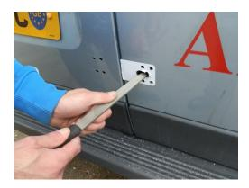
7) Touch up bare metal edges with protective paint.
