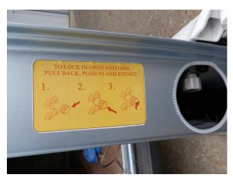
14) Check all fastenings are tight, gaskets correctly placed and lock operation, your lock is now ready for use.
