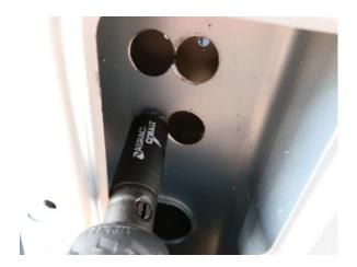
5) In order to access catch mechanism we would recommend a 50-75mm hole subject to vehicle door thickness at 90 degrees to lock. See Photo.
