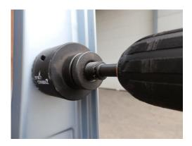
6) Deburr all holes and file away sharp edges, especially 2 x (B) 25.4mm holes.
