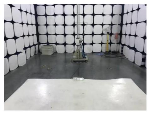
Description: Back View Radiated Emission Test Setup
