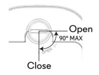
Turn the screw 90 degrees Clockwise to lock the battery cover.
