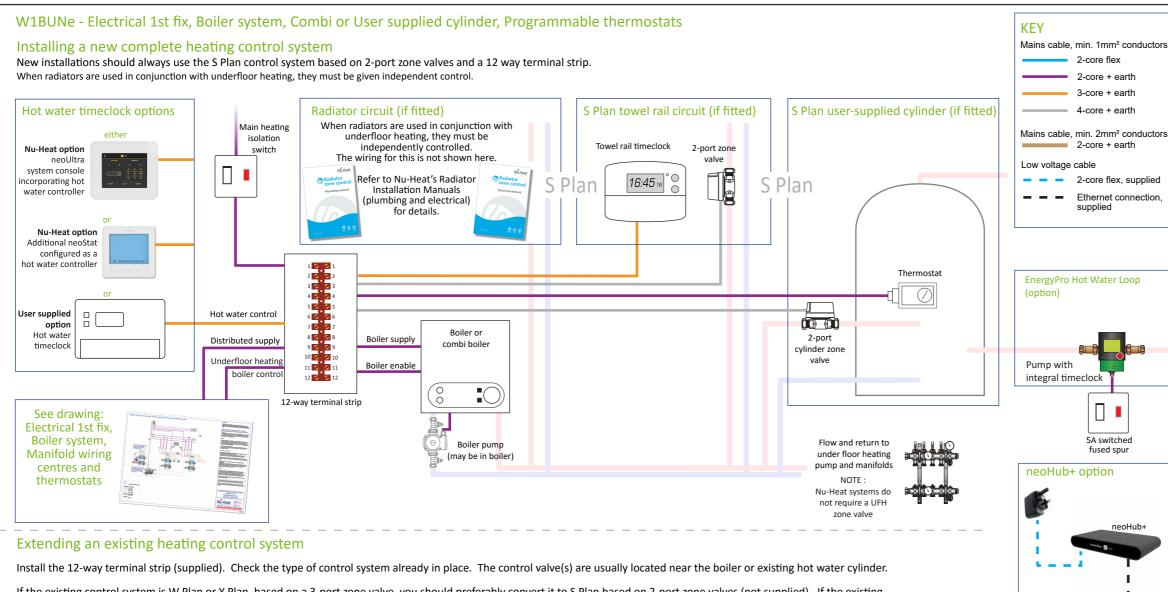
If the existing control system is W Plan or Y Plan, based on a 3-port zone valve, you should preferably convert it to S Plan based on 2-port zone valves (not supplied). If the existing system is based on 2-port zone valves then it is already 'S Plan' so leave the existing zone valves in place. For S Plan you can EITHER leave the installed timeclock in place OR use the designated control (if supplied) to control hot water. See above for 1st fix cabling requirement.
