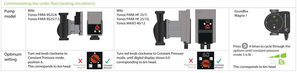
**Underfloor Heating Control System** CHJNil - Commissioning the control system, Heat pump system, User supplied thermostats
