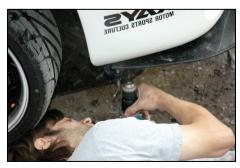
With luck you should be able to get a couple of G-clamps in place to hold the splitter panel to the bumper. If you can do this it is also helpful to support the splitter in the middle to prevent it from 'sagging' between the two clamp points.
