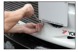
Mark the correct position for the top fastenings using a pencil. Check the alignment both vertically and horizontally to ensure the two tie bars will be symmetrical.
