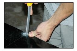
Cut the panel following the line that you scored onto it. Cut slightly outside of the line so that you can rub the cut line smooth. you should attach the top fixings for the tie-bars at this stage, before you restrict access to the reverse of the bumper with the splitter panel.
