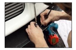
With the tops of the tie-bars in place, align the bottom half of the tie-bar with the panel and put a small mark showing this point. Ensure that both tie-bars are aligned symmetrically.
