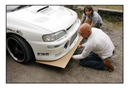
Using a large sheet of cardboard (probably some of the box that the splitter came in), position the cardboard underneath your front bumper and align it so that one edge is at the rearmost point of the front bumper/spoiler.
