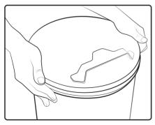
Press down firmly on the lid to make sure it is well seated into the seal.
