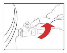
To let air back into the chamber, turn the re-pressuring (inlet) valve on the degassing chamber counter-clockwise into the open (inline) position.
