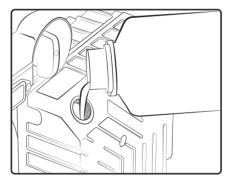
The *LC20EC* pump ships without oil and needs to be filled to the correct level using the supplied oil before use.
