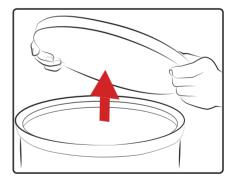
Once air can no longer be heard passing through the filter the chamber will be back up to normal atmospheric pressure.
